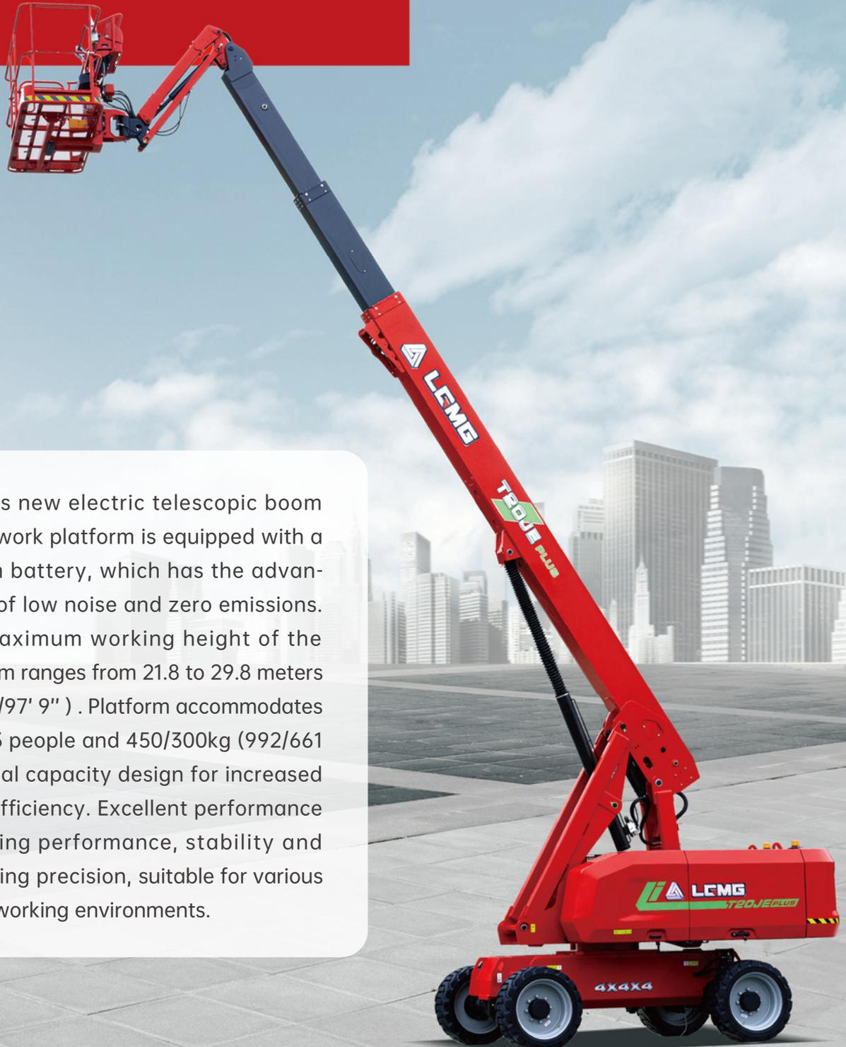
LGMG's new electric telescopic boom aerial work platform is equipped with a lithium battery, which has the advantages of low noise and zero emissions. The maximum working height of the platform ranges from 21.8 to 29.8 meters (71' 6" / 97' 9" ). Platform accommodates up to 3 people and 450/300kg (992/661 lbs) dual capacity design for increased work efficiency. Excellent performance in driving performance, stability and operating precision, suitable for various harsh working environments.
